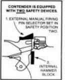
The Contender is equipped with two safety devices which function independently of each other (1. Safety position on the External Manual Firing Pin Selector. 2. Internal Hammer Block). When the Contender action is broken open properly, as explained on pages 5 and 6, the hammer block moves up into a position between the hammer and the frame. In this position the hammer cannot move forward.
